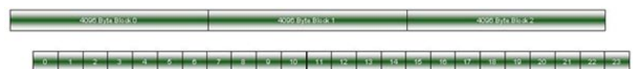
LBA 0 is aligned to the 2 nd 512 byte block of the physical 4K sector = Alignment 1
